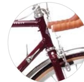
The Clubman Country features additional water bottle mounts & a pump peg. Its centrepull brakes are controlled by traditional levers with gum-rubber hoods, and down tube indexed levers control the 16sp derailleur.
