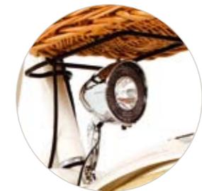
Along with an alloy propstand for ease of parking, a fully fitted lighting set offers added safety with a dynamo operated headlamp and a high visibility mudguard mounted rear light.
