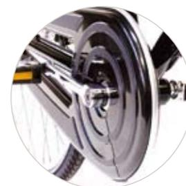
A fully enclosed chaincase protects you and your bike from unwanted grease and grime. This helps to reduce wear and tear on the chain and decreases the amount of maintenance that your bike will require.
