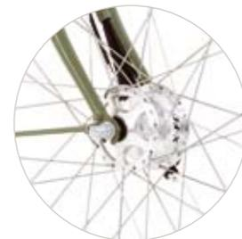
Sturmev Archer alloy hub brakes provide excellent stopping power whatever the weather and are very low maintenance. Add these to wheels with puncture resistant tyres and you have a truly practical machine.
