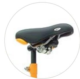
The Pickle is fitted with a child-specific padded saddle on an L-shaped seat post. The post's unique shape allows the tricycle to be adjusted to fit as your child grows.
