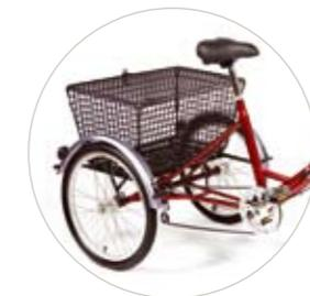
The Tri-1 features a large rear platform for the attachment of bags or boxes. As an optional accessory, a capacious wire basket with a hinged top is available which can be locked with a small padlock. This basket is ideal for shopping and/or recycling trips.
