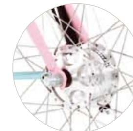
The Tube Rider features alloy brake hubs to give you the stopping power you need come rain or shine. Built on to high quality alloy rims with stainless spokes, this wheel combination is built to last.
