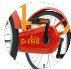
To protect inquisitive fingers from the chain the Pickle is fitted with a fully enclosed chaincase. This also helps to keep out dirt and water, reducing wear on the sheltered components.
