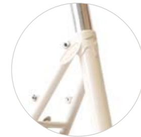
The frame is hand-made with lightweight Reynolds 531 tubing – the original ‘standard of excellence’ in frame building – and combines modern geometry with a slender step through design using fine lugged construction.
