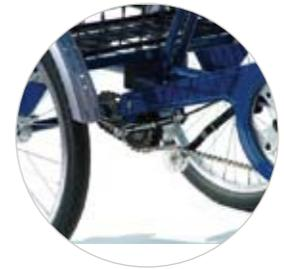
The three speed hub gear system provides both easy shifting low range gears and ease of maintenance. The gears can be changed whilst stationary which allows for the perfect getaway from junctions.
