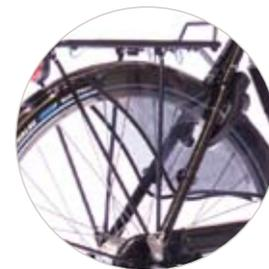
The Princess features rear skirtguards integrated with the hand-lined mudguards to provide all season practicality and comfort. Additionally, the Sovereign model features a multi-tube alloy rack for added luggage support.
